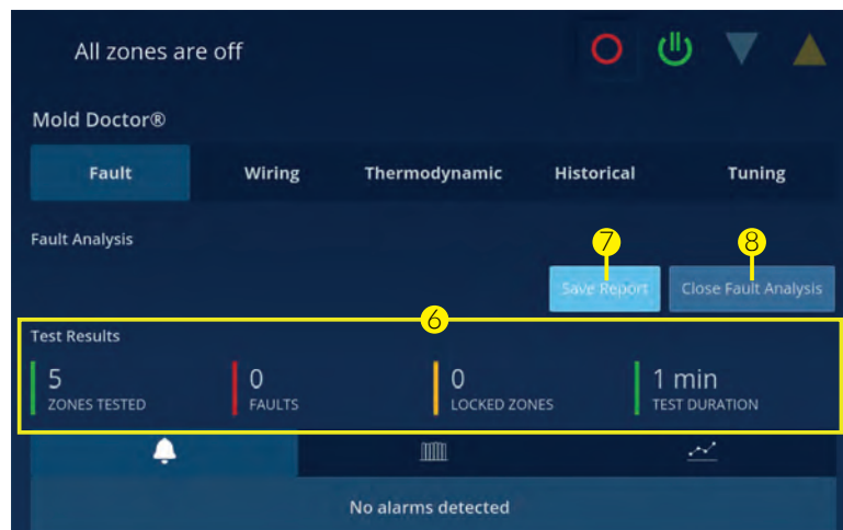
Fig. 88 Mold Doctor - Fault Analysis Completed
