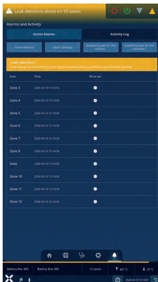
Fig. 64 Alarm Page - Leak Detection Alarm
