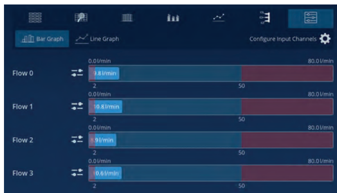
Fig. 123 Analog Inputs Alarms Active
